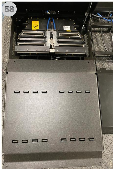
26. To close the lid of the sensor housing, you must pull the pin on the safety catch.
