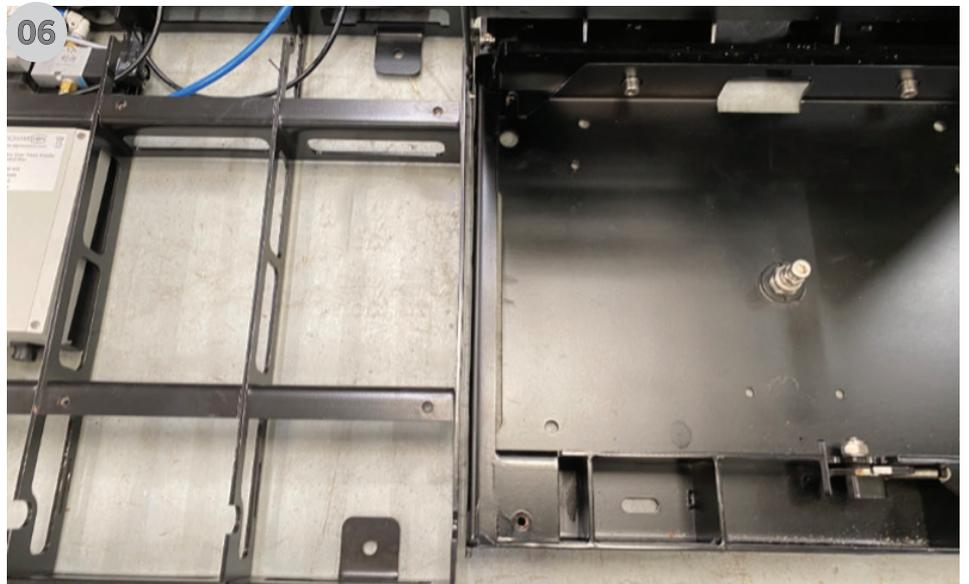
11. Fix the sensor housings to the floor, use four fixings for each housing.
