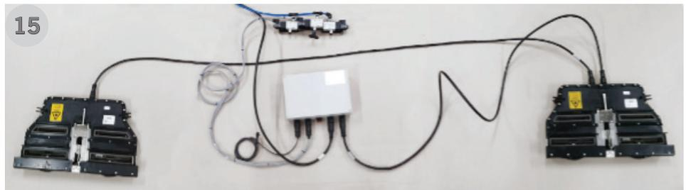
16. Route the main air supply to the solenoid block. This supply should be filtered and regulated 8-10bar.
