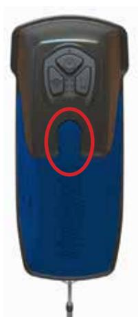
The scanner has a built in rechargeable Li-Ion battery, that can be charged with supplied 5VDC 2A USB charger. A fully charged scanner will usually last a full working day.
