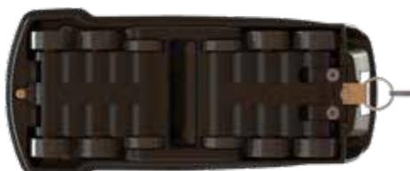
To clean the optical window, release the wheel assembly on the underside of the scanner by pushing the two retaining clips. This allows the wheel assembly to pivot on a hinge away from the base of the scanner.
