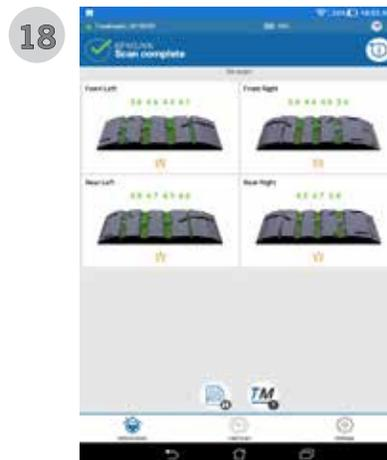
When landing on the 4 scan page, the **TREADMANAGER™** icon will upload any scans completed.
